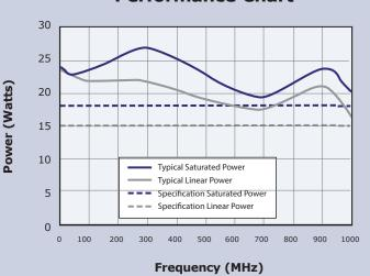
Choose **GaAs Class A** for the ultimate in linearity, ruggedness, efficiency and cost - only from Vectawave.
